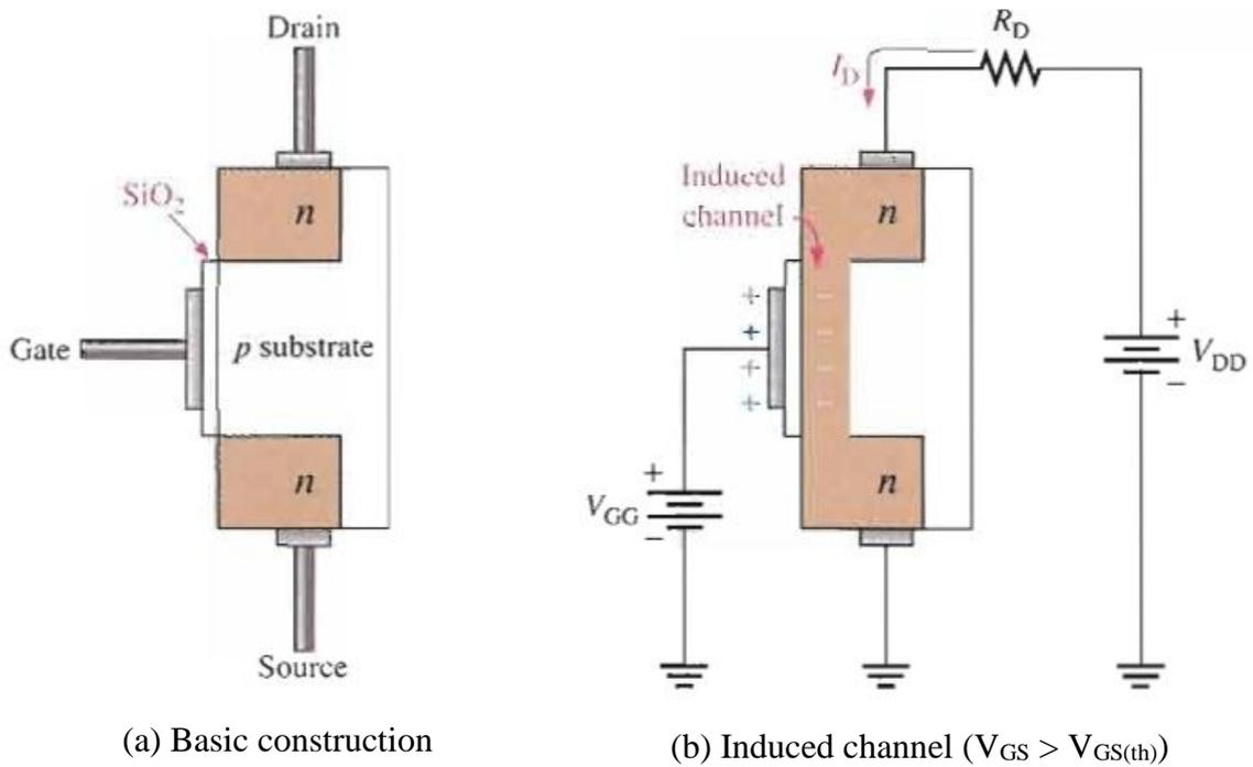
Figure (18): The basic E-MOSFET construction and operation (n-channel)
