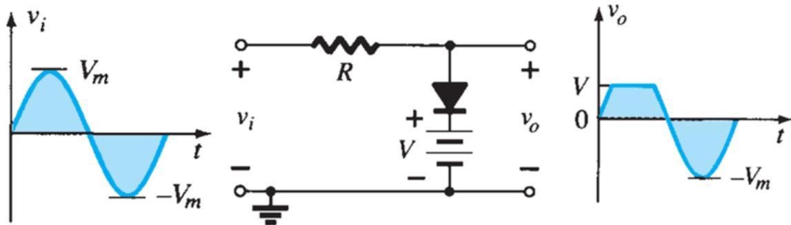
Figure (24): Clipper operation
