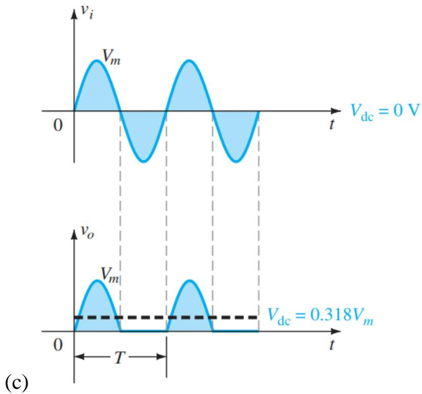
Figure (12): Half-wave rectifier operation
