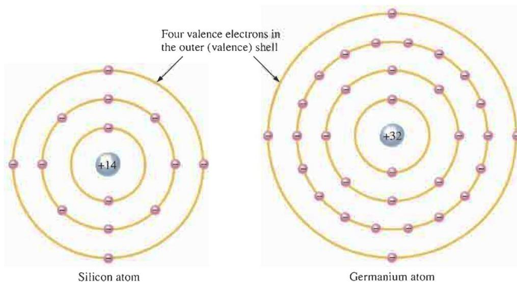
Figure (2): The Silicon and Germanium atoms
