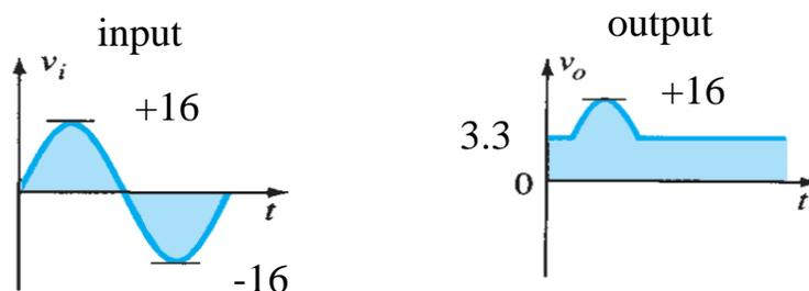
Figure (24) shows another shape forming in the clipper circuit that the diode will be in the “on” state for a portion of the positive region of the input signal. When the diode is in its short-circuit state the output voltage will be directly across the
