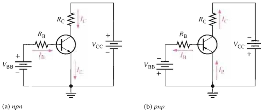
Figure (5) a) npn; and b) pnp circuits
