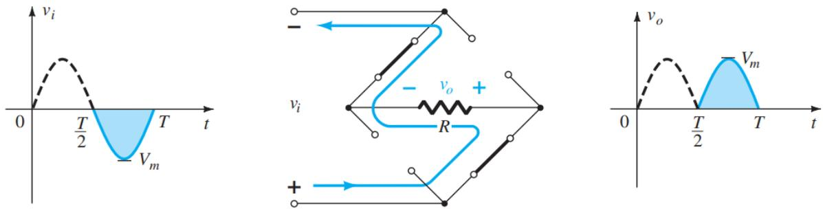
Figure (15): Full-wave rectifier operation (second stage)
