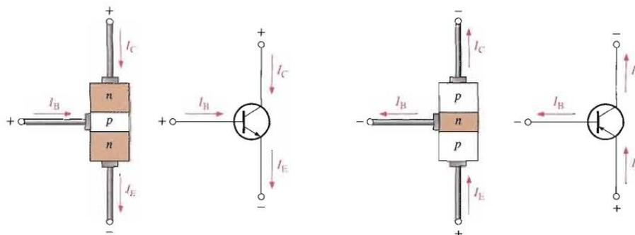
Figure (4): Transistor current flow
