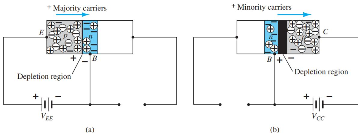
Figure (2): Biasing a transistor: (a) forward-bias; (b) reverse-bias
