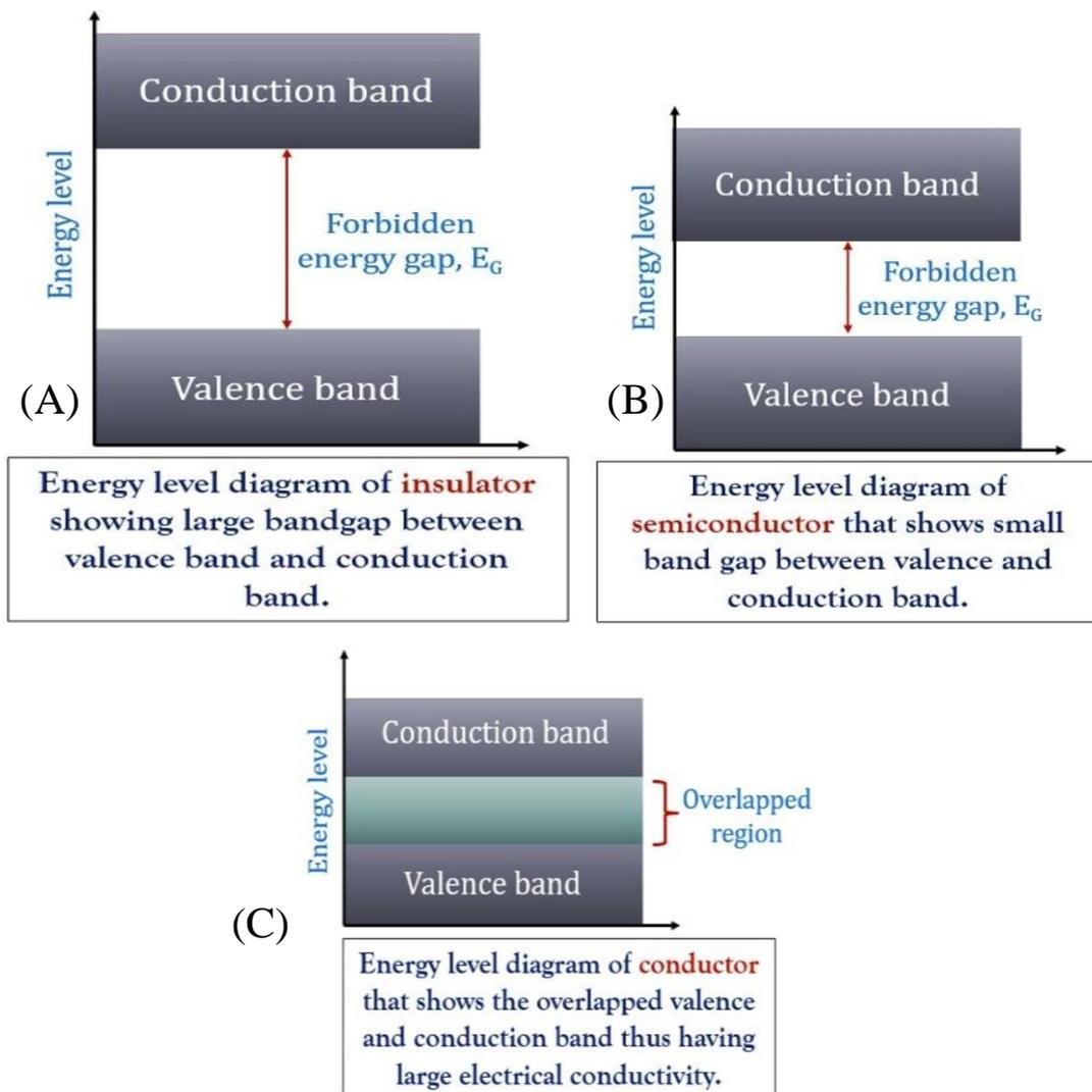
Figure (1): The energy level diagram of A) insulator, B) semiconductor, C) conductor
