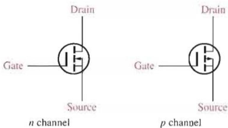
Figure (19): E-MOSFET schematic symbols
