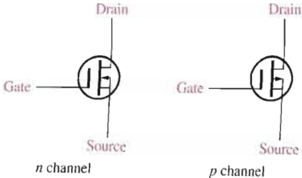
Figure (17): D-MOSFET schematic symbols
