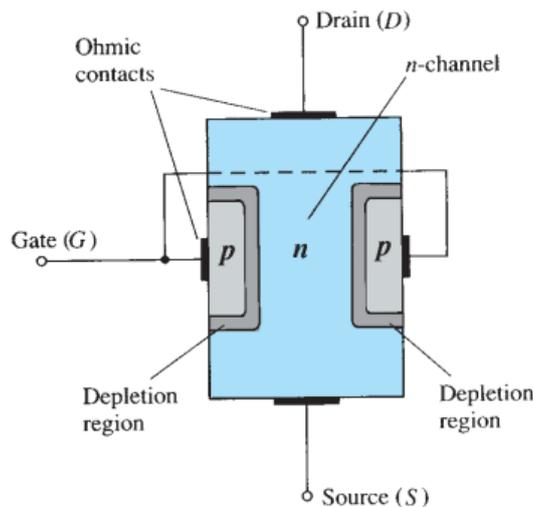
Figure (9): Junction field-effect transistor (JFET).
