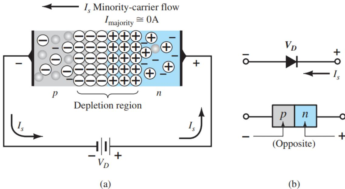
Figure (7): Reverse-biased p–n junction: (a) internal distribution of charge under reverse-bias conditions; (b) reverse-bias polarity and direction of reverse saturation current.
