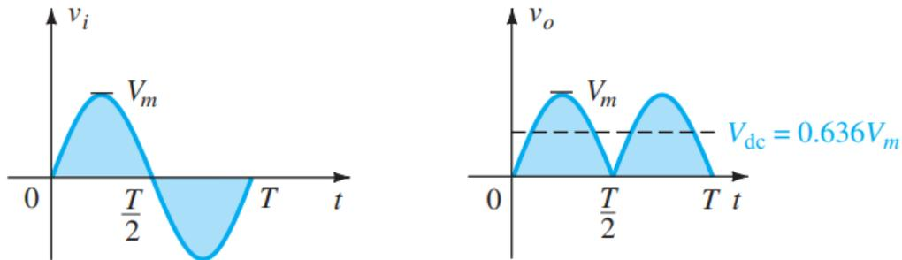
Figure (16): The input and output waveforms for a full-wave rectifier
