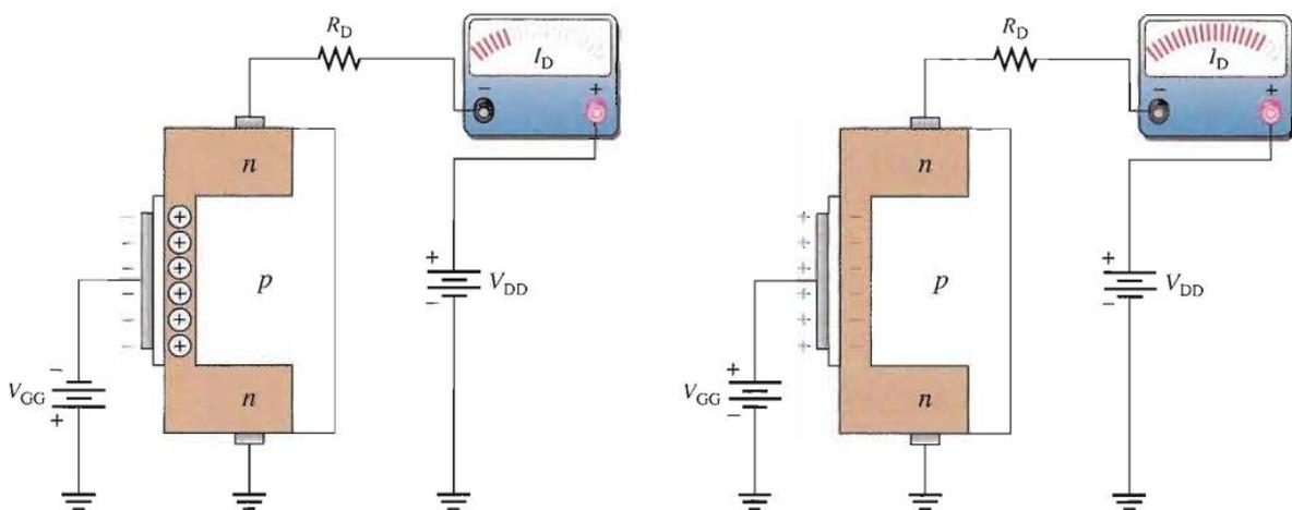
(a) Depletion mode:  $V_{GS}$  negative and less than  $V_{GS(off)}$     (b) Enhancement mode:  $V_{GS}$  positive
