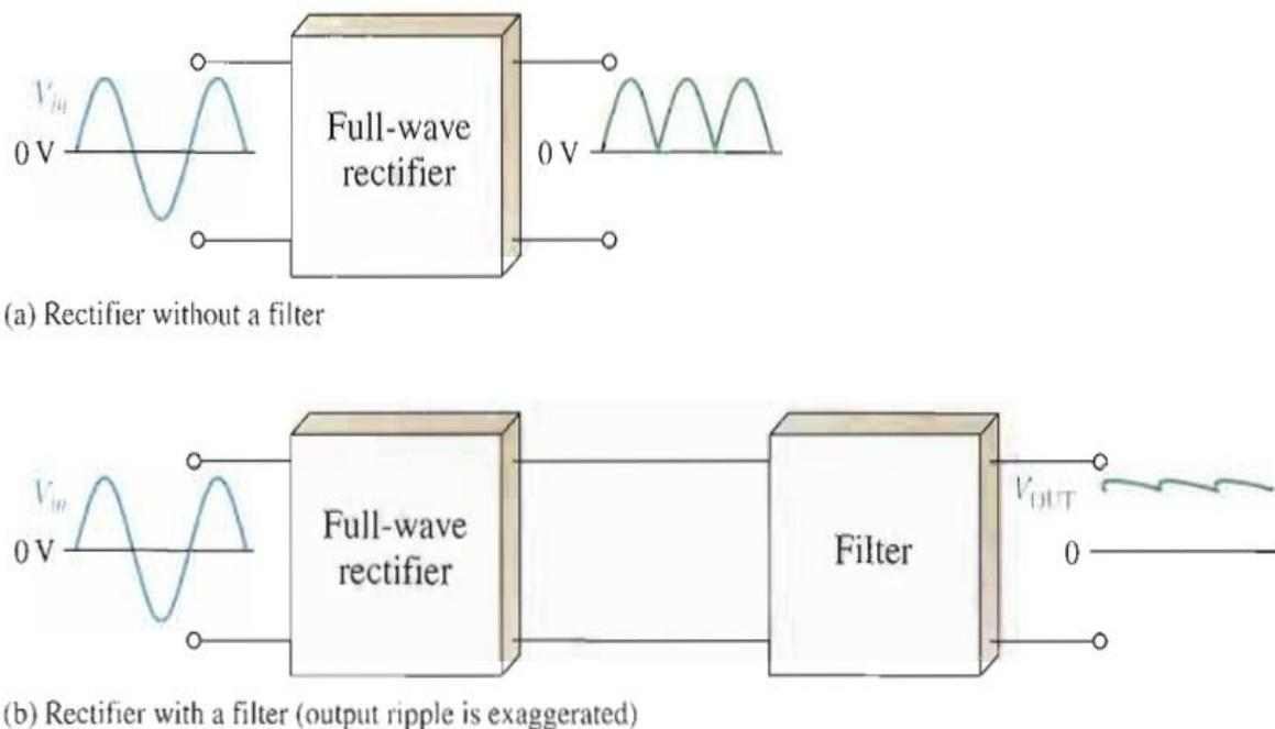
Figure (17): The filtering concept
