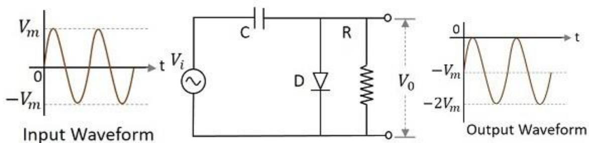
Figure (25): Negative Clamper circuit operation
