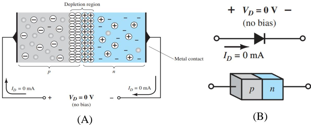
Figure (6): A p–n junction with no external bias: (A) an internal distribution of charge; (B) a diode symbol, with the defined polarity and the current direction
