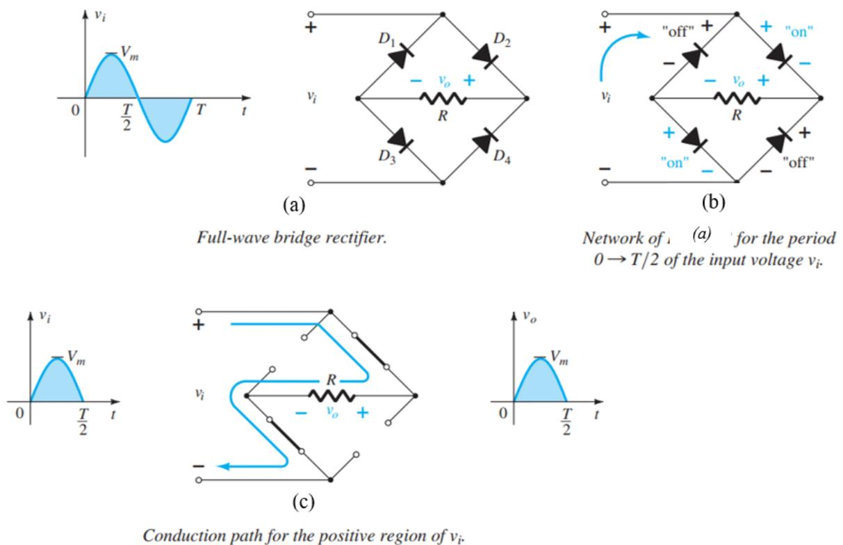
Figure (14): Full-wave rectifier operation (first stage)
