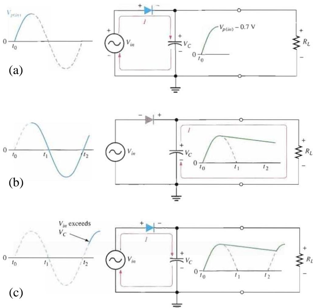
Figure (18): Half-wave rectifier with capacitor operation
