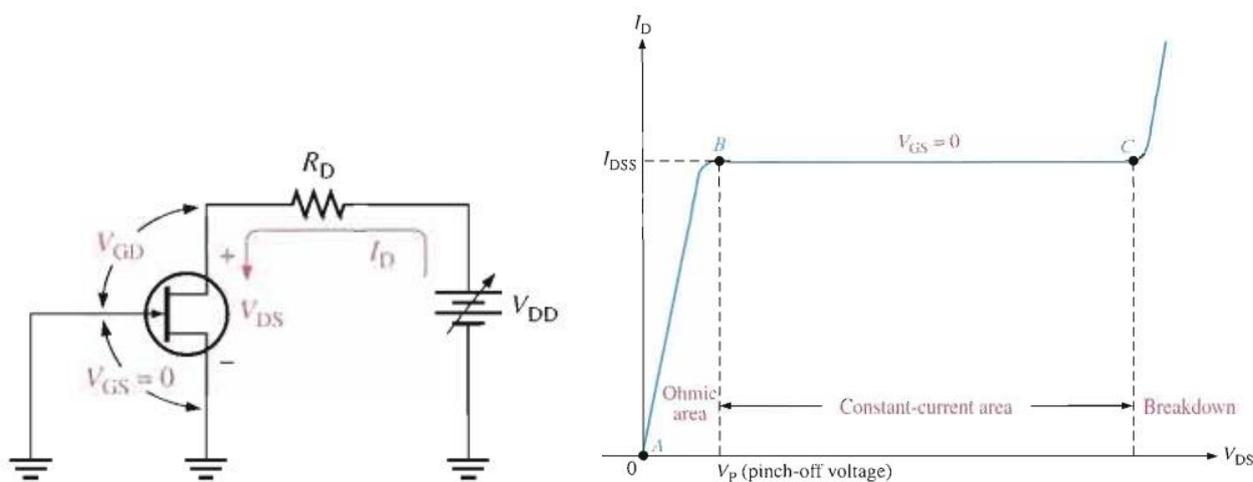
(a) JFET with  $V_{GS} = 0V$  and variable  $V_{DS}$  ( $V_{DD}$ )
