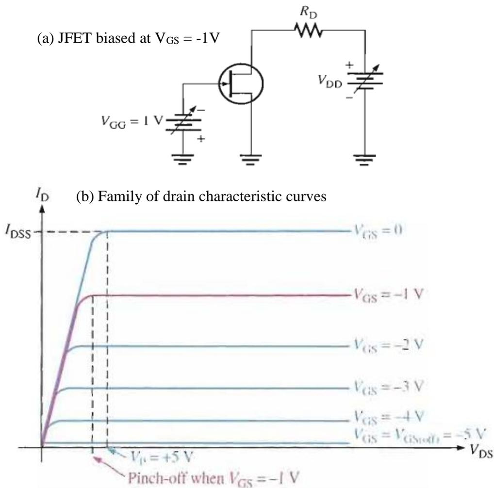
Figure (14): Pinch-off occurs at a lower  $V_{DS}$  as  $V_{GS}$  is increased to more negative values
