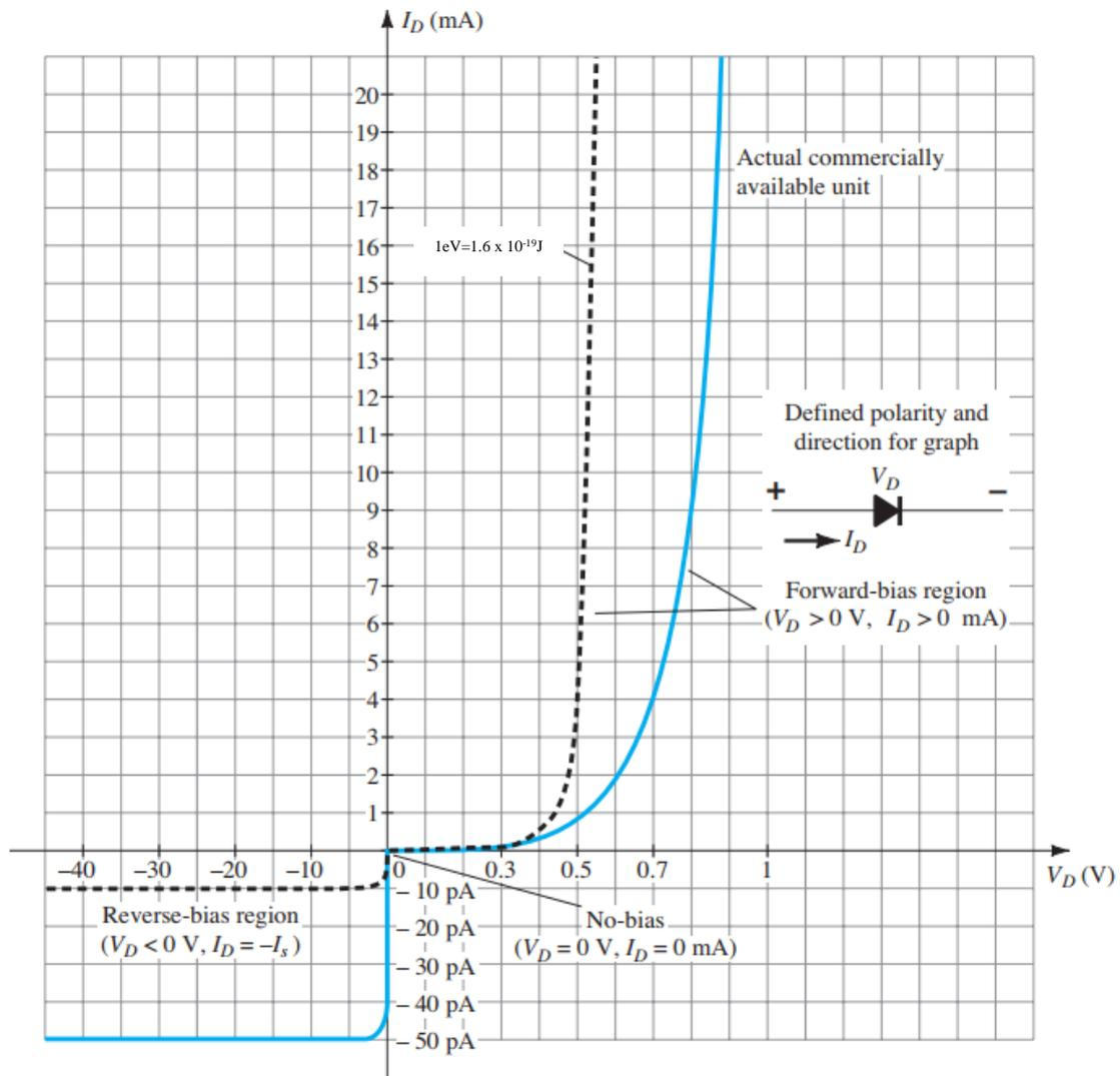
Figure (9): Diode Characteristic
