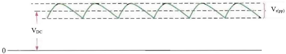
Figure (22): The calculation of the ripple factor
