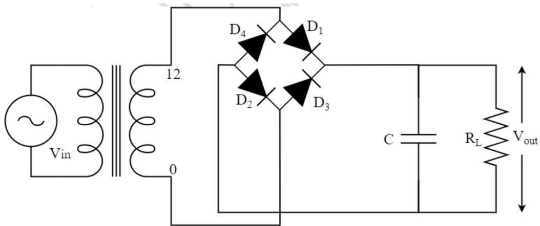
Figure (20): Full-wave rectifier with capacitor
