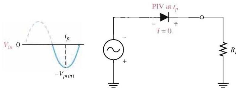
Figure (13): The PIV occurs at the peak of each half-cycle of the input
