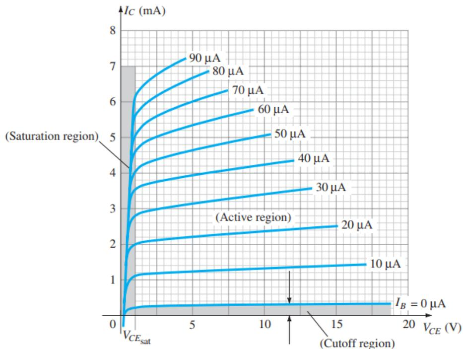
Figure (8): Collector Characteristic curve
