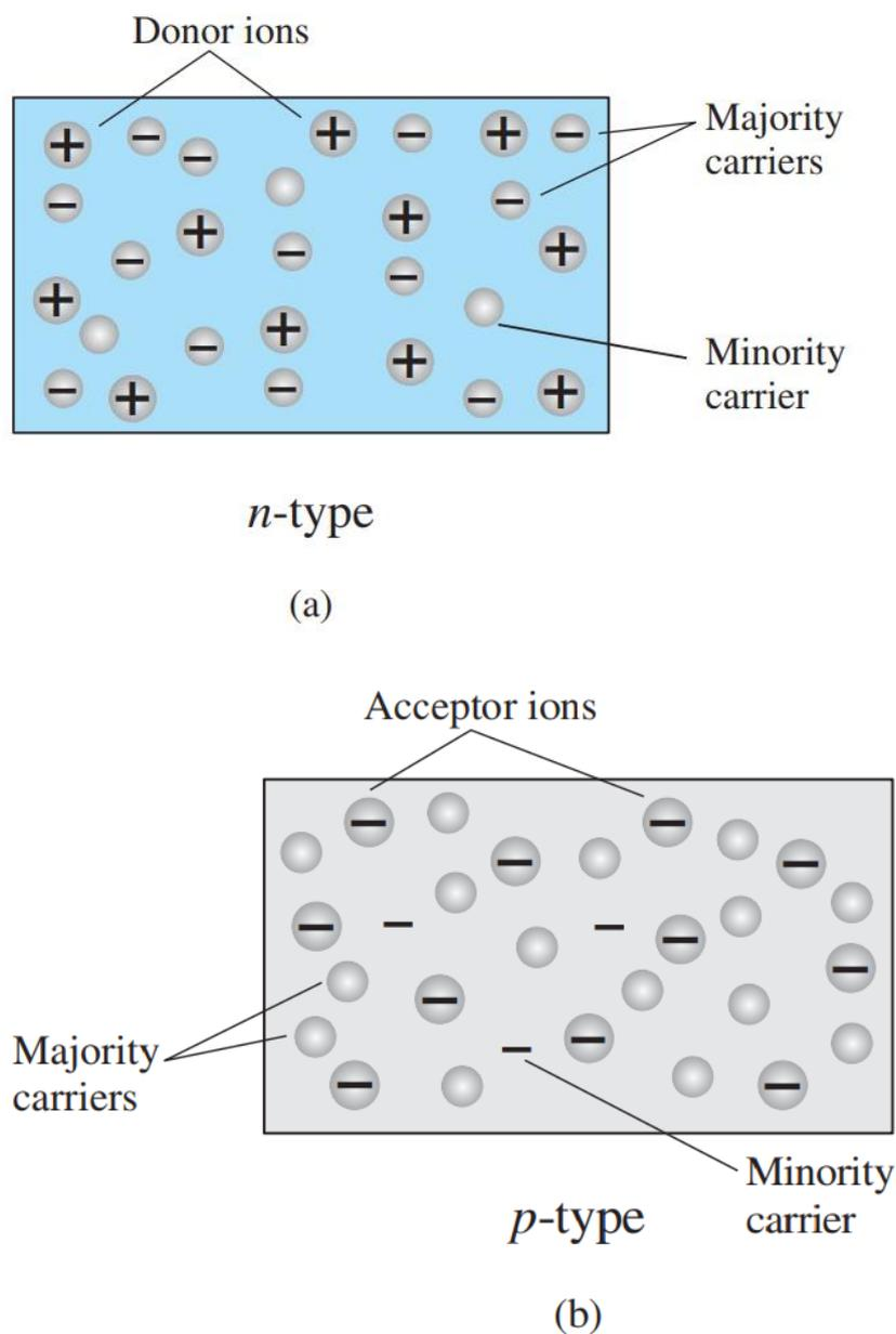
Figure (5): (a) n-type material; (b) p-type material.
