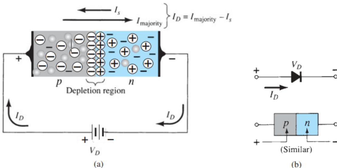
Figure (8): Forward-biased p–n junction: (a) internal distribution of charge under forward-bias conditions; (b) forward-bias polarity and direction of resulting current
