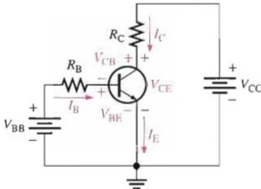
Figure (6): Transistor currents and voltages
