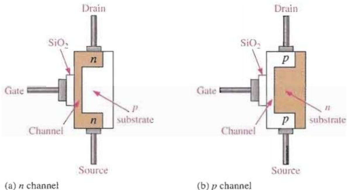
Figure (15): Basic structure of D-MOSFETs
