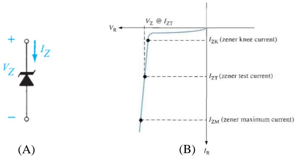
Figure (11): A) The symbol, and B) The reverse characteristic of a zener diode
