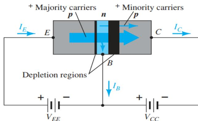
Figure (3): Majority and minority carrier flow of a pnp transistor
