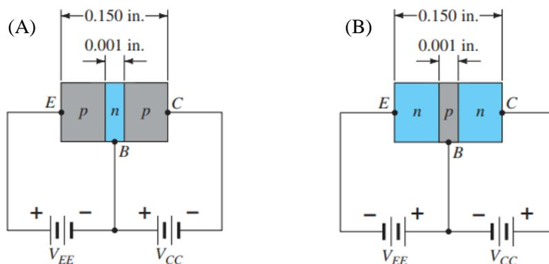
Figure (1): Types of transistors: (A) pnp; (B) npn
