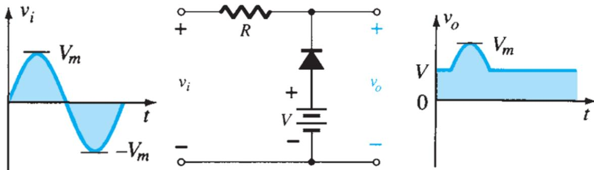
Figure (23): Clipper operation
