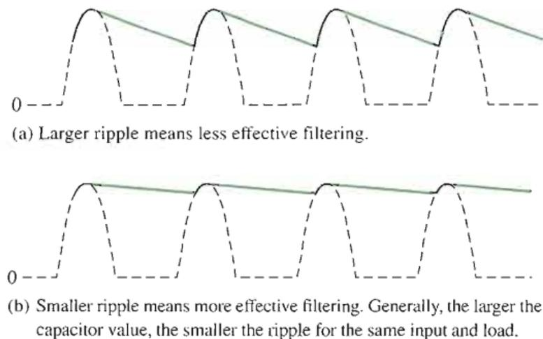
Figure (19): Half-wave ripple voltage waveform
