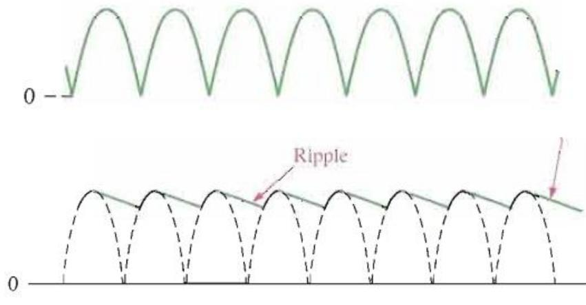
Figure (21): Full-wave ripple voltage waveform
