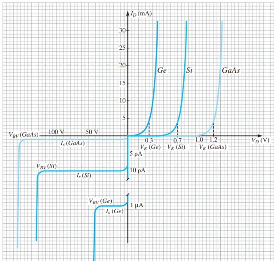
Figure (10): Comparison of Ge, Si, and GaAs commercial diodes
